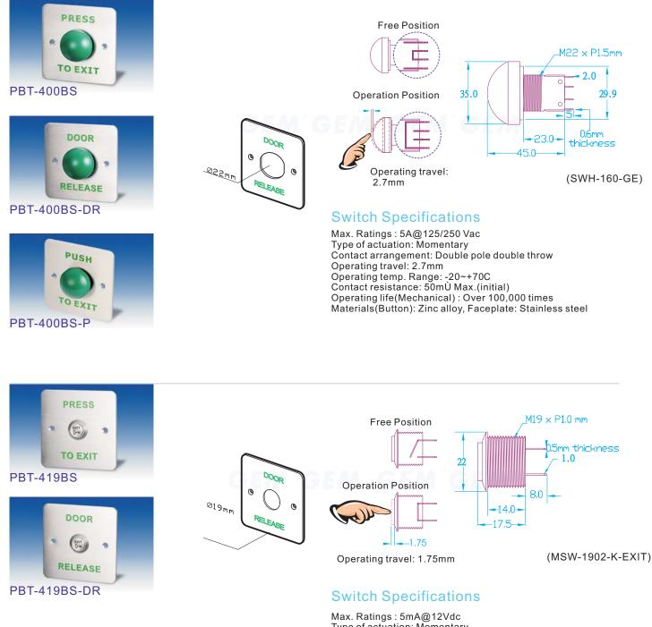
Type of actuation: Momentary Contact arrangement: Single pole single throw (N.O.) Operating travel: 1.75mm Operating temp. Range: -20~+70C Contact resistance: 1kÙ Max.(initial) Operating life(5mA 5Vdc): Over 100,000 times Materials: Stainless steel
